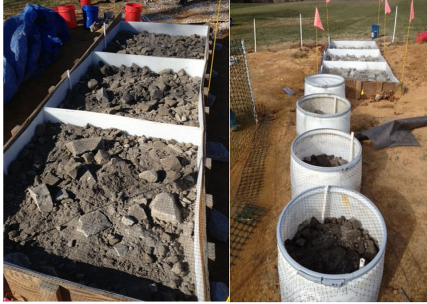
Figure 6. Harlan spoil leaching mesocosms (left) and barrels (right foreground) at Virginia Tech Turfgrass Research Center (VTRC) in November 2012. Leachates were collected monthly or following significant precipitation events and analyzed for pH and specific conductance. Ion composition was also monitored periodically (only 2021 data reported here).
