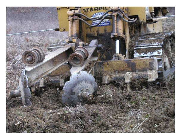
Photo 1. An advanced ripping tool used to prepare the biomass research sites by Union Concrete Products of Maxwelton, West Virginia, under the direction of J. K. Rose.
