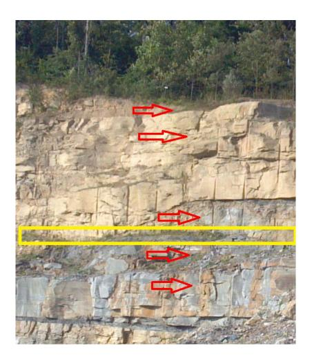
**Figure 1** – An example profile illustrating the field sampling scheme employed. Each distinct layer (red arrows) is collected and described. Special notice of the boundary between brown and gray materials (yellow box) is also taken, in an effort to better characterize the transition between these materials. Of the 24 samples to date, this boundary is often a tight shale layer or thin coal seam.
