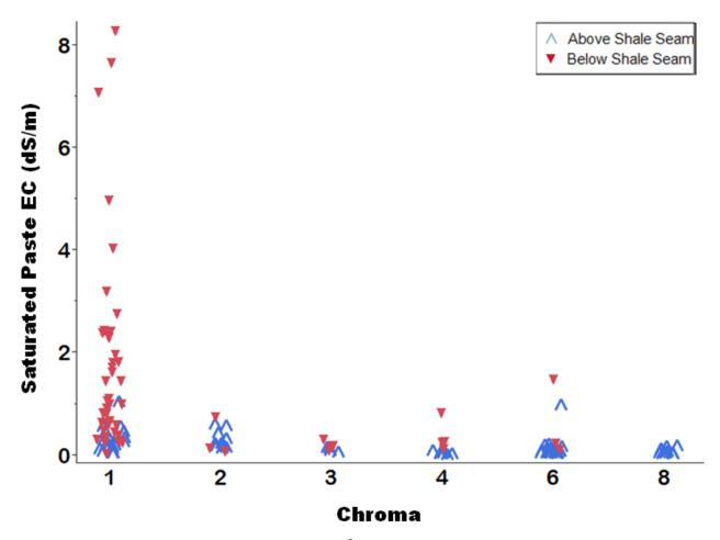
**Figure 5-** Saturated paste EC versus Munsell<sup>©</sup> color chart "chroma" recorded for moist samples. Lower chromas represent darker, grayer samples. The colors represent the lowest chroma present in the case of mixed matrix colors.
