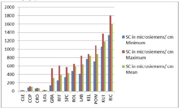
**Figure 3:** Specific conductance values at study sites, reported by Timpano (2011). Sites were chosen along a gradient of specific conductance. The four streams with mean SC < 200  $\mu$ S/cm are reference streams.
