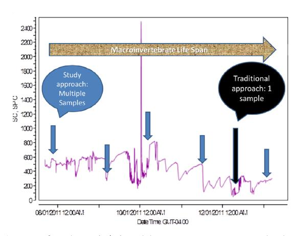
Figure 1: Specific Conductance ( $\mu$ S/cm) recorded every 15 minutes in Spruce Pine Creek, with traditional point-in-time sampling and study approach with multiple samples.
